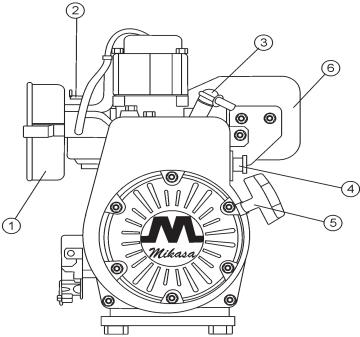
Figure 2. Engine Controls and Components
